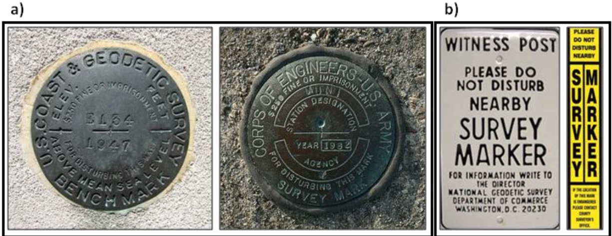
Figure 10. Examples of: a) metal disk survey benchmarks, and b) witness post label, established by USACE and NGS.
