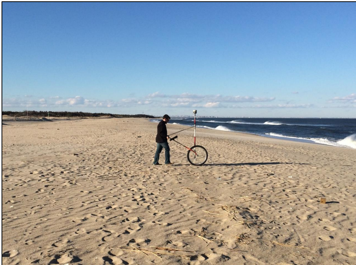
Figure 13. Survey wheel constructed to facilitate the efficient collection of 3D topographic data.
