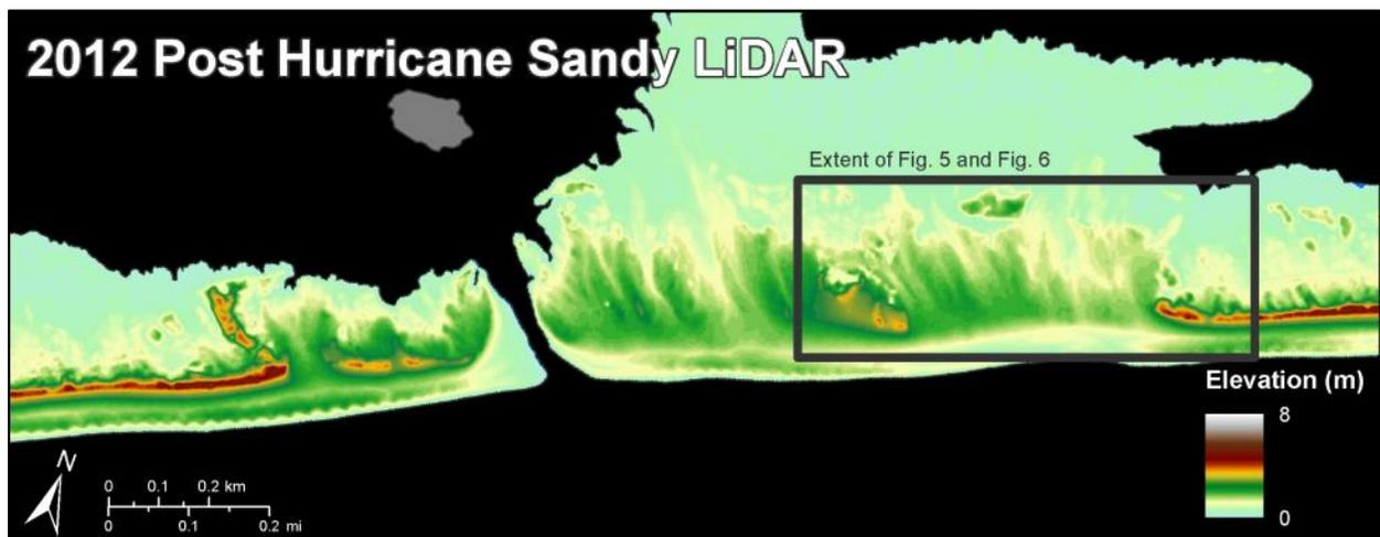
**Figure 3.** Digital elevation model (DEM) with elevation categories created from 2012 Post Hurricane Sandy LiDAR data set with reduced point density, Otis G. Pike Wilderness Area, Fire Island National Seashore (Data available through USGS (Woolpert, 2012)). Inset window identifies location of the area incorporated in Figures 5 and 6.
